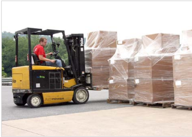
Fuel cell-powered forklift at work (Susquehanna)
