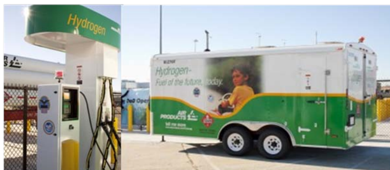
DLA Distribution Warner Robins, GA's stationary and mobile hydrogen refuelers
