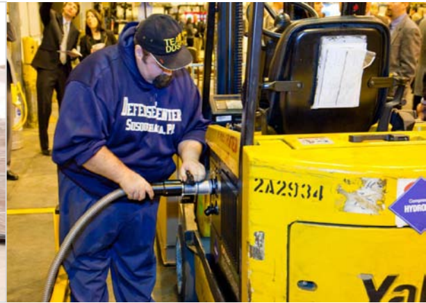
Fuel cell forklift being refueled at one of Susquehanna's two indoor hydrogen dispensers
