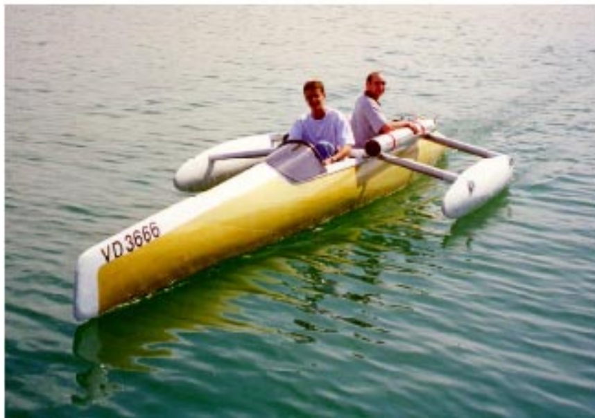
Fig 2 PEFC propelled boat « Hydroxy300 » 300W – 12 km/h.
